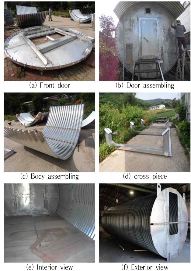
Figure 2. Manufacturing the cast-in-place structures using corrugated metal-plates
